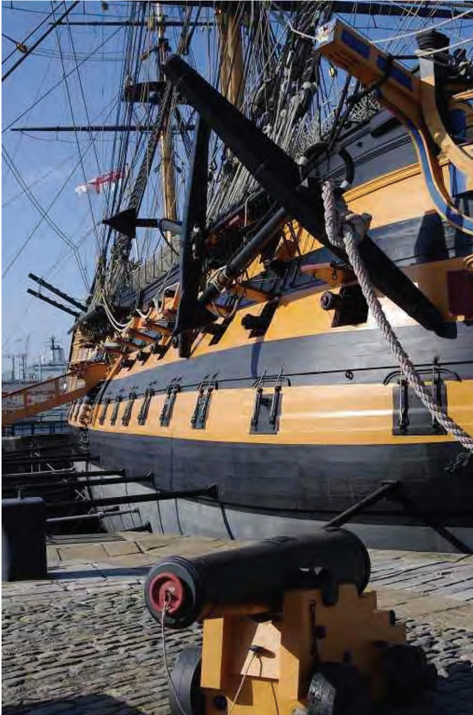
Figure 5: HMS Victory in dry dock at Portsmouth Dockyard, showing the complex rigging and guns mounted on three decks (© The Author).
